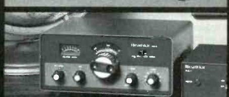
Microelectronics make the new HW-9 QRP CW transceiver small and light.
